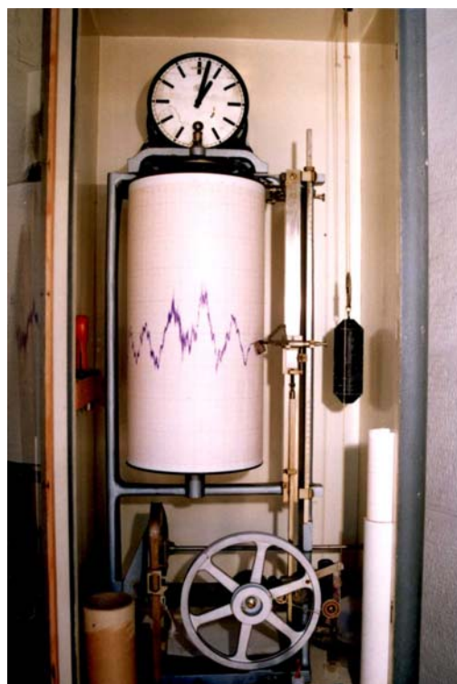
Fig. 2 Mechanical tide-gauge A. Ott – Kempten at Split.
