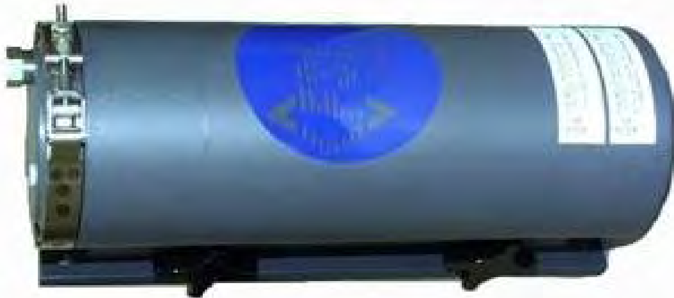
General sight of the tide gauge
