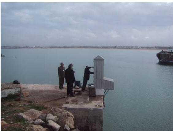
Figure 22, Mohammedia Port Radar Tide Gauge
