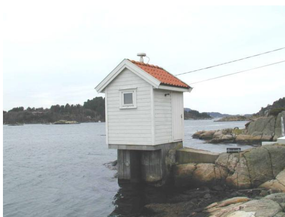
Figure 2. Tide gauges with continuous GNSS receivers at Tregde (to the left) and at Andenes.
