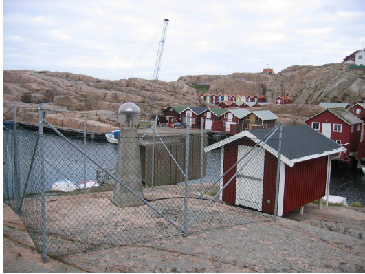
Figure 4. Smögen, a mareograph (hut in the background) also combined with CGPS (monument in the front) and absolute gravity platform (hut to the right).
