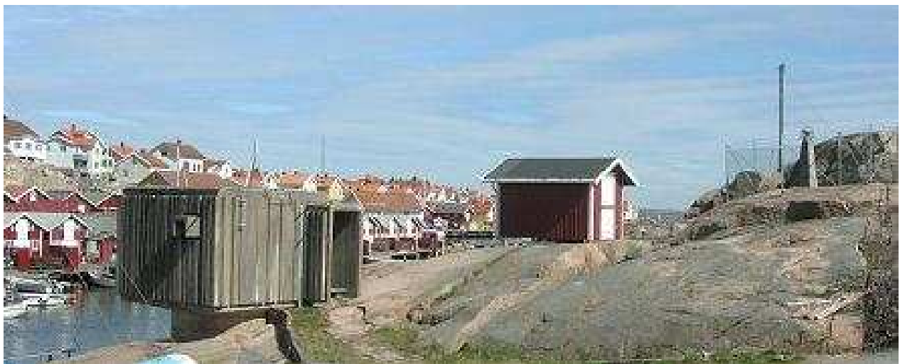
Figure 5. Smögen, a mareograph (hut to the left) also combined with CGPS (monument to the right) and absolute gravity platform (hut in the middle).
