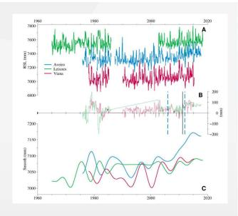
B. Differences between the raw time series for each TG with respect to Aveiro. The black solid vertical line marks the epoch corresponding to a possible discontinuity in the time series for Aveiro; the blue dashed vertical lines mark the epochs corresponding to a change of equipment in Aveiro (we cannot exclude the turning point to be related with the change of equipment. In any case, caution is required in the interpretation of the trend for this tide gauge.)
