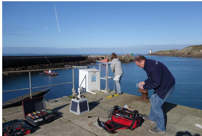
Mobile Tide Gauge being installed (credit: Shom)
