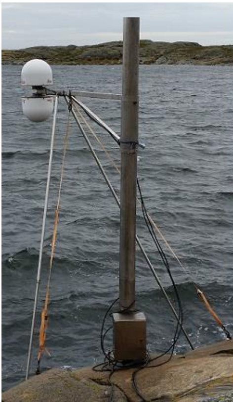
Figure 9. An upward- and downward looking GNSS-reflectometer
