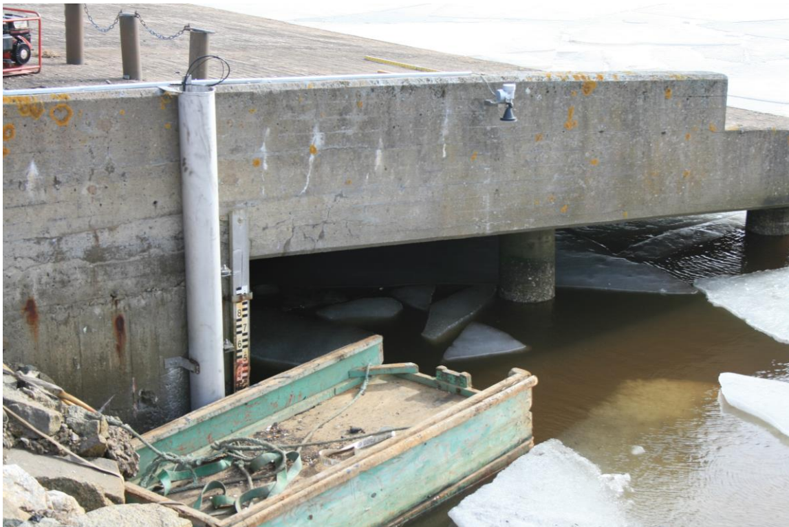
Figure 10. A mobile sea level station, which consists of a bubble-sensor (to the left) and radar sensor (to the right). During periods with ice conditions, the data from the radar sensor are neglected.
