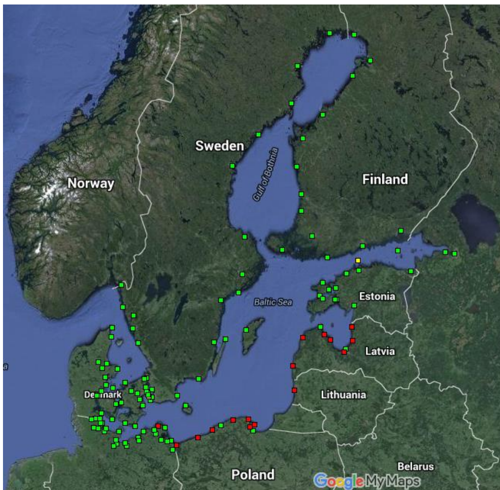
Figure 6. Sea level stations available through the BOOS Community. Stations marked in green are available in near real time. Stations marked in red are not available of different reasons.
