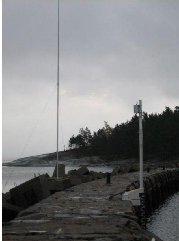
Fig. 1. The above-water part of the autonomous sea-level gauge system at the Hogland Island in the Baltic Sea with the input unit for recording hydrographic information from submerged sensors and transmitting it to servers in St. Petersburg and Moscow via cellular communication.
