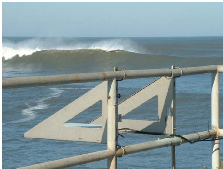
Figure 13. The Miros SM094 sensor at a USACE testing facility.
