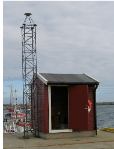
Figure 2: Tide gauges with continuous GNSS receivers at Tregde (to the left) and at Andenes (right)
