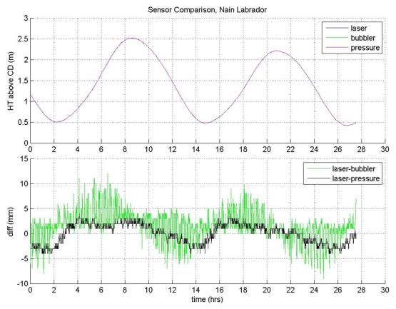
Figure 8: Sensor Comparison at Nain
