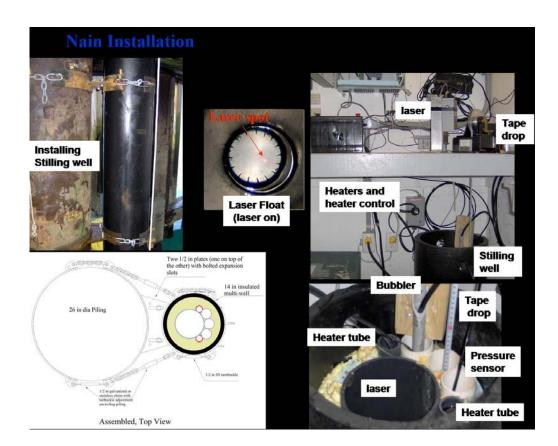
Figure 7: Nain, An Example Installation
