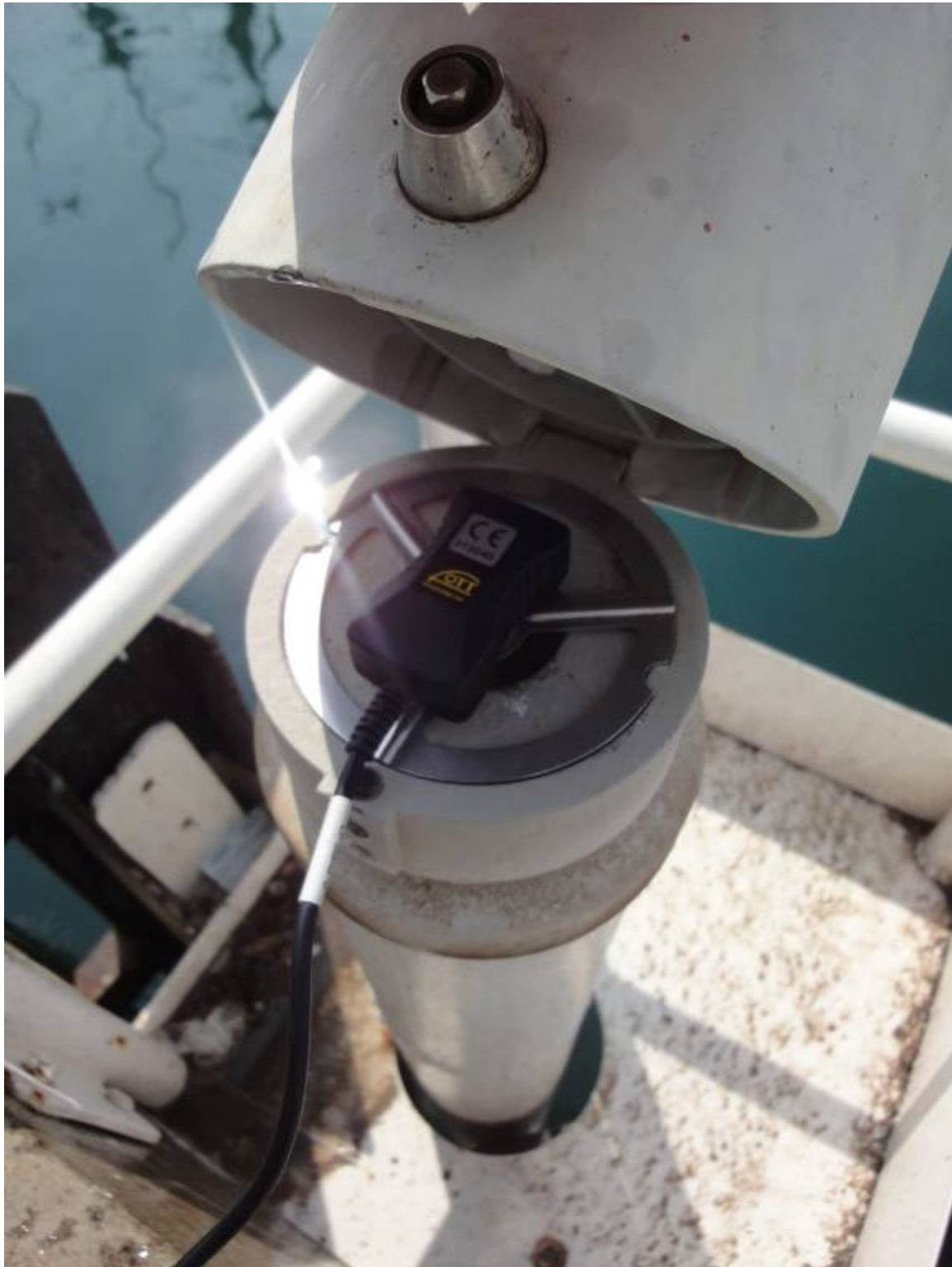
Control port on top of OTT pressure sensor assembly
