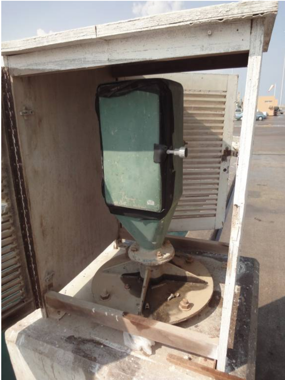
OTT float-based mechanical chart recorder
