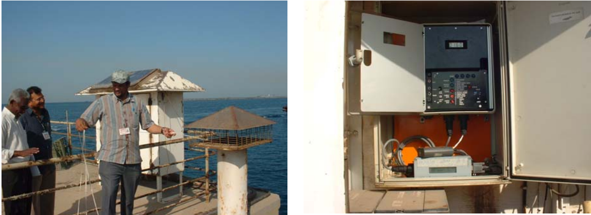
Figure 2: Example of a tide gauge deployed by ARAMCO in the Red Sea. Here it is the Jeddah station.
