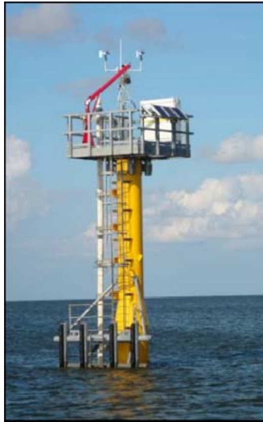
Figure 9. One of the US NOAA Sentinel Tide Stations in the Gulf of Mexico.
